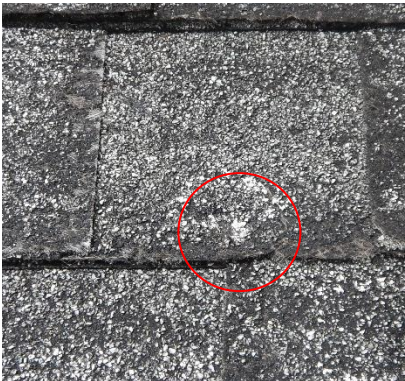
Deck A Hail Test Single Lap
