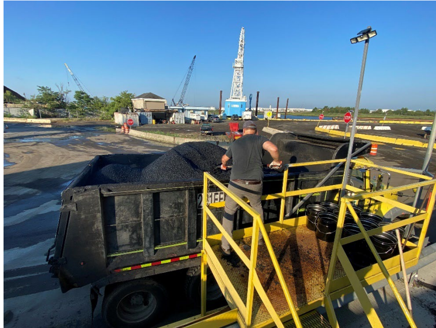
Figure 4 – Sampling Loose Mix from Delivery Truck at Sampling Stand
