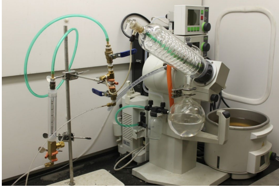
Figure 8 – Asphalt Binder Recovery Equipment at Rutgers University
